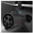
Securely push the adapter into the charging port
